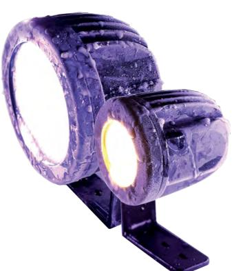
Procolors are in IP67 - IK09 protection class and with their robust and durable structure, are designed to meet extremely difficult requirements of outdoor facade applications. Procolors are resistant to impact, vibration and other harsh conditions, with their aluminum housing and special filler materials. They have passed Verification and Reliability tests.
